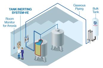
• TANK INERTING SYSTEM-VEM is suitable for inerting up to 60 tanks using electronic offset units connected to one master control unit.
